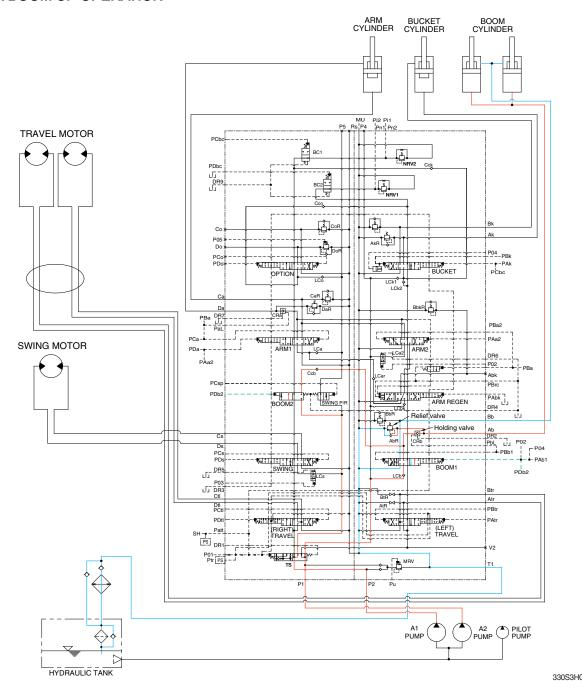
When the right control lever is pulled back, the boom spools in the main control valve are moved to the up position by the pilot oil pressure from the remote control valve.
