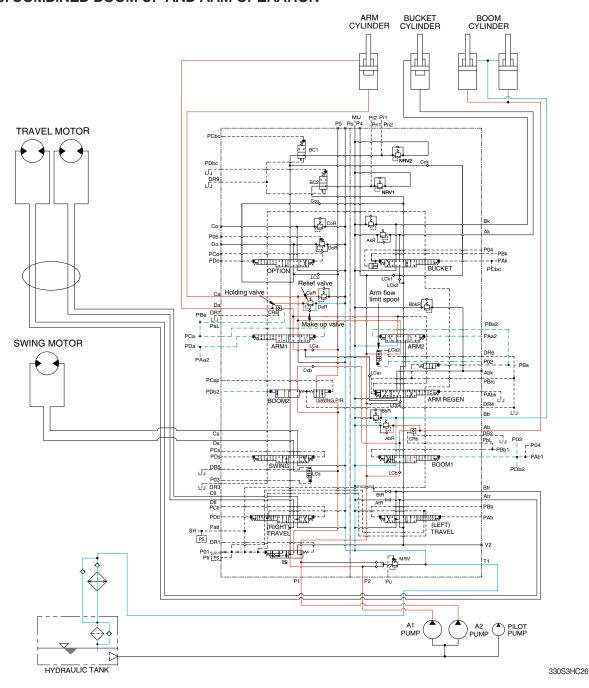
When the boom up and arm functions are operated, simultaneously each spool in the main control valve is moved to the functional position by the pilot oil pressure from the remote control valve.
